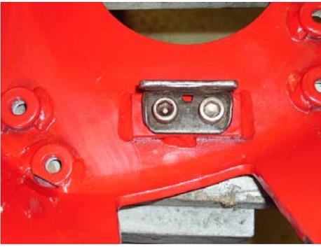
13. Install the Lakewood Bell Housing and secure with all the bolts that came with the purchase. Now you can re-install the Starter also.
