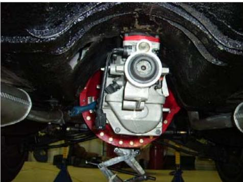
17. Lower the Tremec using the scissors jack until you can re-install the shifter mechanism using a thin coat of silicone for gasket material and secure with the six bolts using loc-tight on the threads. Raise the transmission back in place using scissors jack. The 57 Fairlane doesn't need the tunnel raised for this swap.
