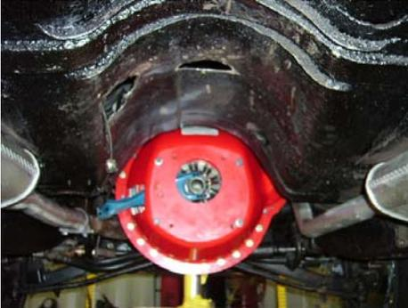
14. Measure the distance from the housing face of the transmission to the shifter locating you're going to use. Then measure that length from the bell housing face and cut a round hole in the transmission tunnel for the shifter to stick through. Make the hole just large enough for the shifter to work without having too large a hole.
