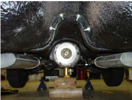
4. Now you can remove transmission cross member and then remove the old transmission using the floor jack and platform.
