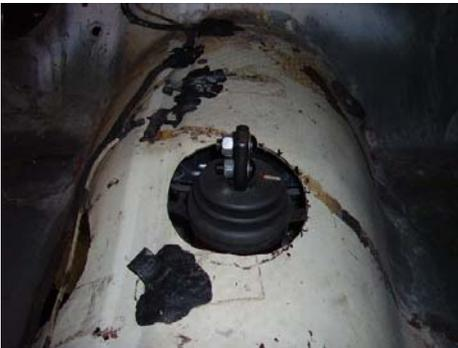
15. Remove the six bolts from the shifter housing of the new TREMEC transmission. Remove the housing. Cover the hole with a clean cloth and tape it into position so dirt can't get in.
